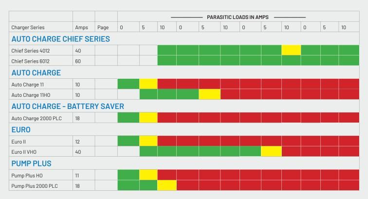
These chargers are for average recharge rates and average sized batteries. For specific applications, please contact our sales or engineering department with battery size, parasitic loads and required recharge time.
